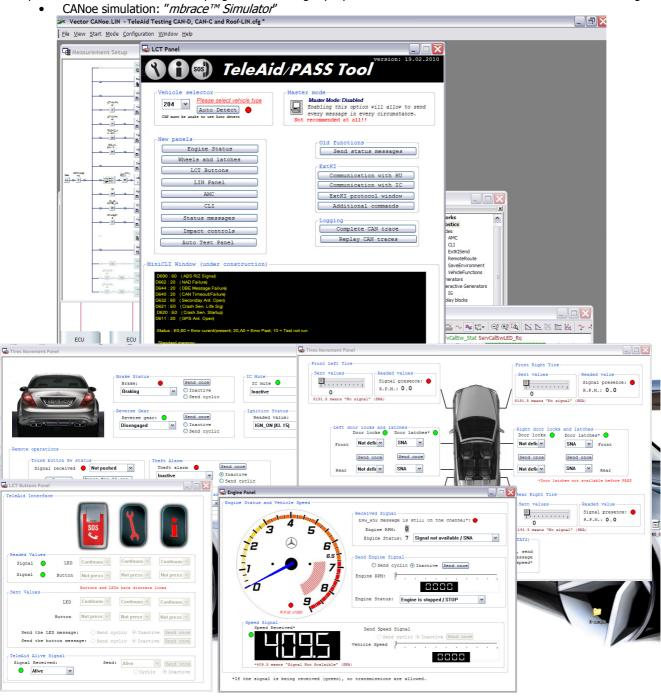
CANoe is an intuitive tool which handles the different signals in the car and lets the user interact with them. It can be programmed with CAPL language and it can handle complex user-machine interfaces that are easy to develop thanks to the included WYSIWYG software. It is usually used for manual testing of the different Electronic Control Units (ECUs) when reproducing any possible use case. Also basic automated testing routines were programmed.
