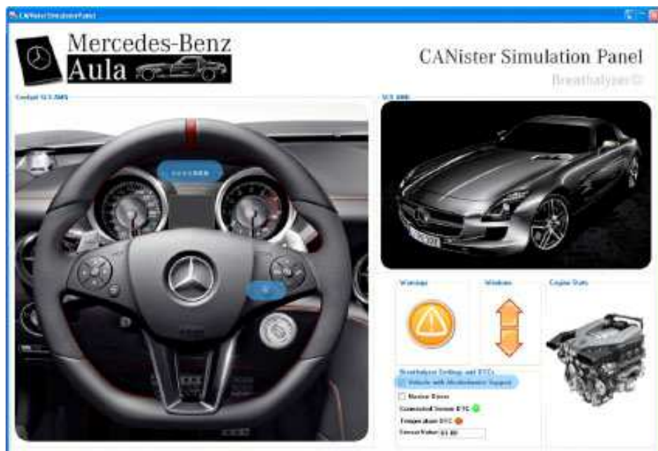
CANoe/CAPL Simulation Panel which interacts with a breathalyser on an external CANister device
