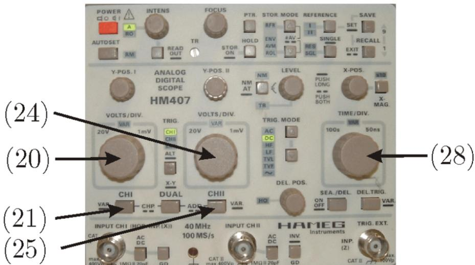
(20) VOLTS/DIV 1, (21) CH 1, (24) VOLTS/DIV 2, (25) CH 2 y (28) TIME/DIV.
