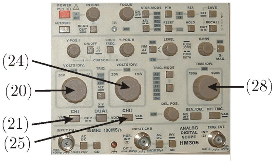
(20) VOLTS/DIV 1, (21) CH 1, (24) VOLTS/DIV 2, (25) CH 2 y (28) TIME/DIV.
