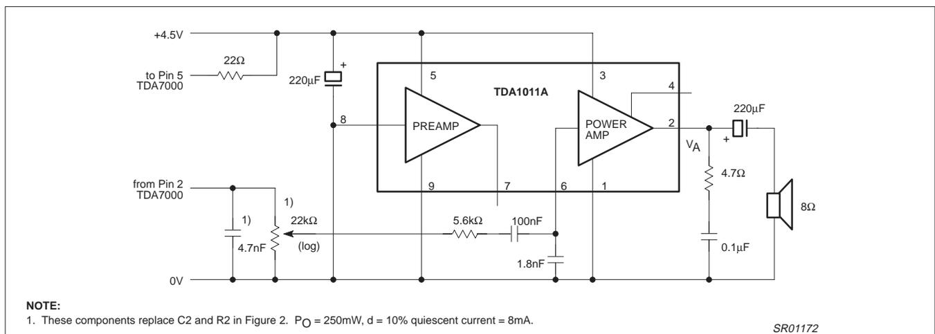
**Figure 19. An Integrated 250mW Audio Output Stage**
