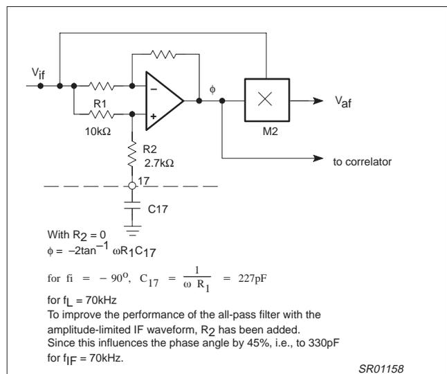
Figure 5. FM Demodulator Phase Shift Circuit (All-Pass Filter)
