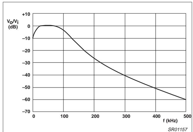
Figure 4. Measured Response of the IF Filter
