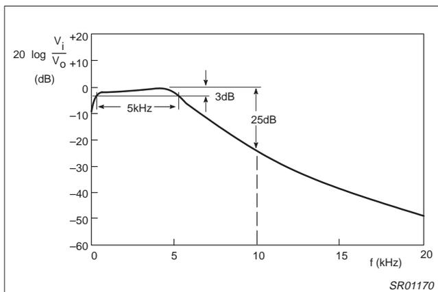
Figure 17. IF Selectivity for the Narrowband FM Receiver
